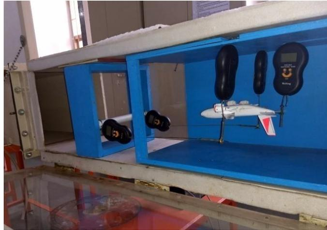
Fig. 7. Model with force sensors inside the test section
