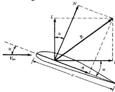
Fig. 2. Components of the aerodynamic force [5]
