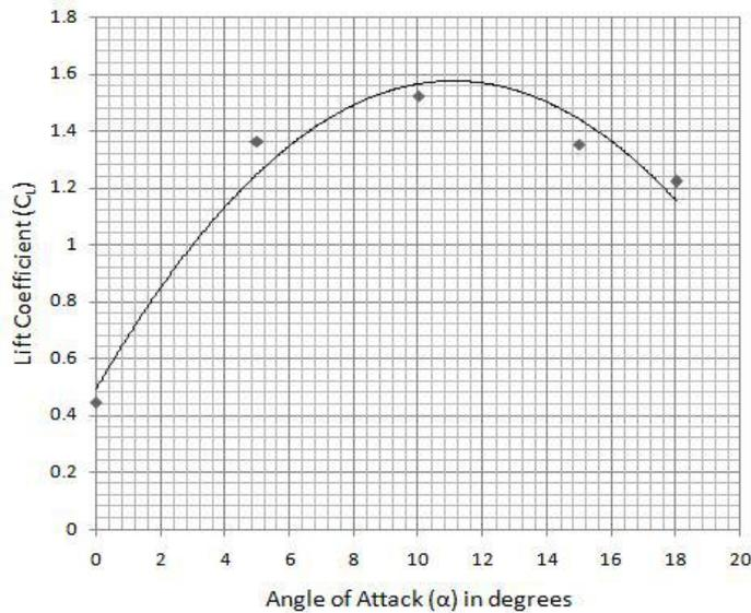
Fig. 8. Lift Coefficient Vs Angle of Attack
